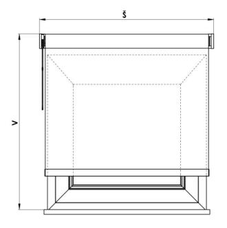
The blind can be positioned into or in front of the hole (on the ceiling or the wall).
